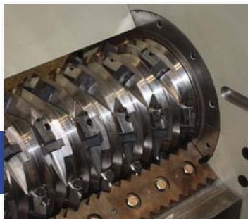
self-cleaning rotor seals
