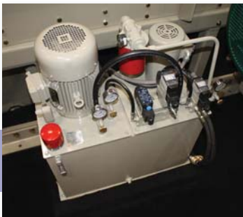
dual pump hydraulic ram
